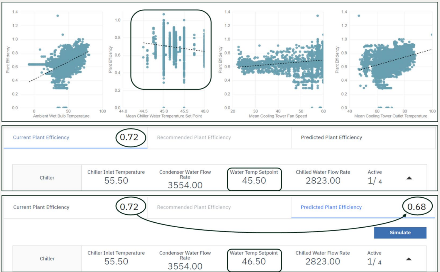
Figure 6: Simulation of new setpoint values not based on historical data
